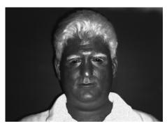
The Tactical Imager for Night/Day Extended-Range Surveillance (TINDERS) is a tactical imaging system that can covertly track and zoom in on a face hundreds of meters away, capture an image, and identify a person through computer face recognition, in the light of day or the dark of night.
