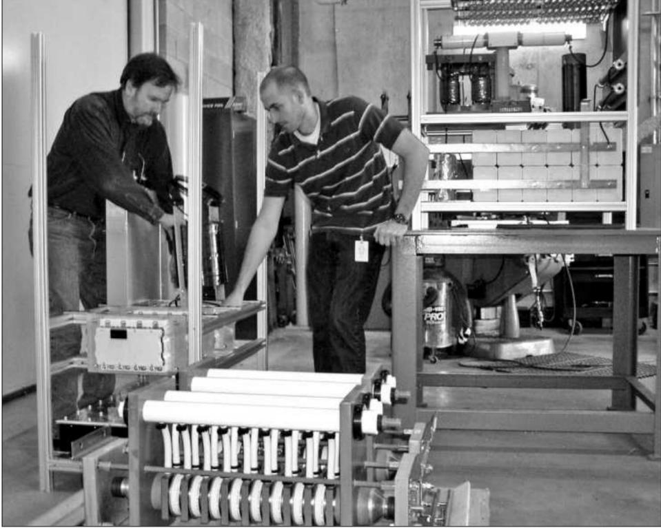
(LEFT) Members of the WVHTC Advanced Technologies Group are pictured assembling a research prototype for an ultra-compact high-power transformer that could be used to help communities following a disaster.
